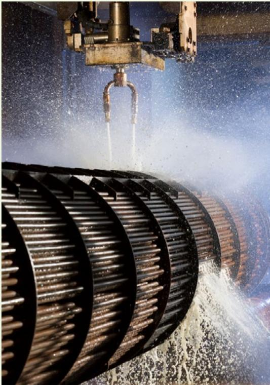
In 2011, Ohmstede Ltd., a part of EMCOR Industrial Services, developed an innovative, environmentally friendly process for cleaning heat exchangers used in refinery and chemical plants, capable of conserving massive amounts of water. Since then, the Ohmstede team has cleaned over 5,000 heat exchangers equating to 3.5 million tubes.
